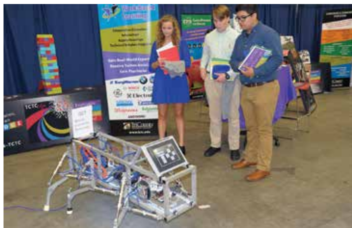
Students from the Pickens County Career and Technology Center observe a Hexapod, a six-legged walking machine powered by pneumatics, controlled by a PLC and built by General Engineering Technology students.
